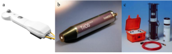
Fig. 2. Radiometers used in the observation. a. CNR4, b. Ramses ACC-VIS, and c. PRR800/810.
