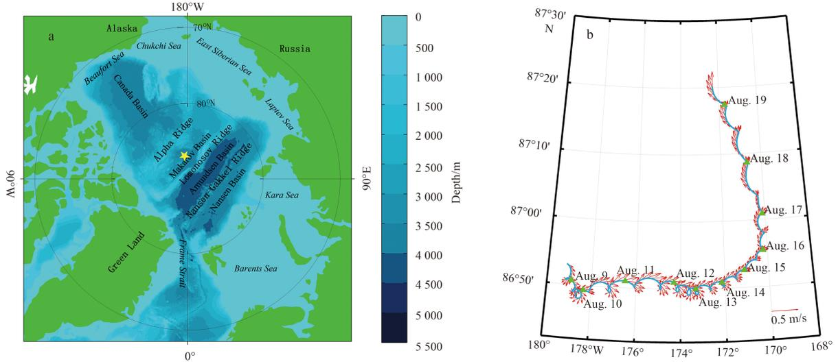
**Fig. 2.** Bathymetric map of the Arctic Ocean and central location of the ice camp (designated by yellow pentagram) (a); and trajectory of the ice camp (b), the starting location of the ice camp for each day is designated by green triangles, hourly mean drifting velocity by red arrows.
